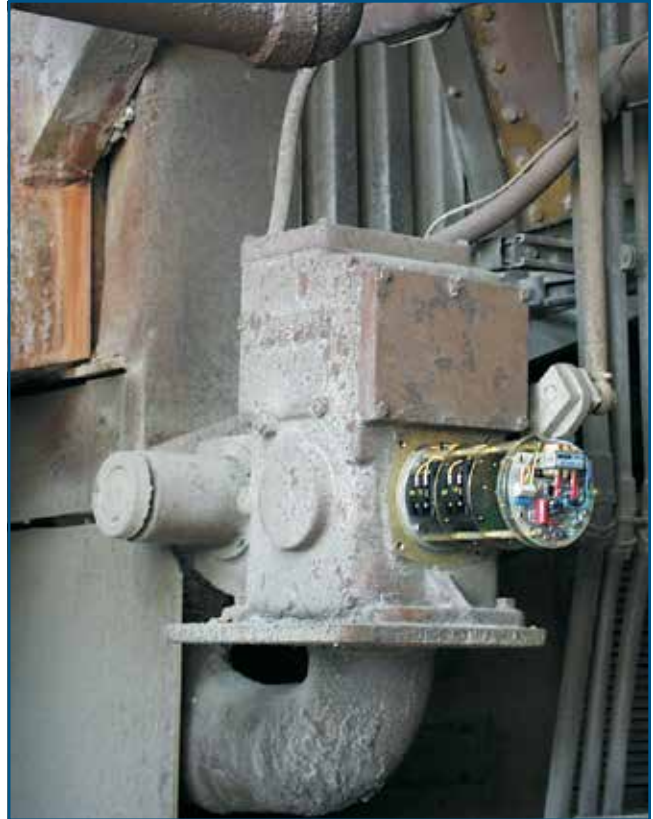
Individual compartments protect components
