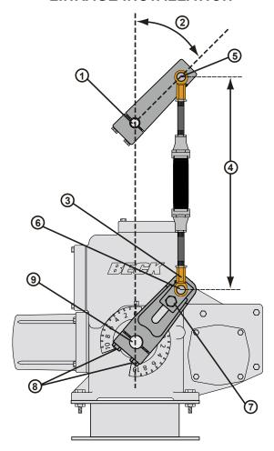
To adjust the linkage length, it is preferable to use the stud couplings. The couplings have right-hand and left-hand threads, so it is not necessary to disconnect the ends to make a length adjustment. Be careful not to expose more than 7" (178 mm) of stud between the rod end and coupling.
