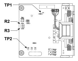
Low Voltage 24 V dc Relay Board Components
