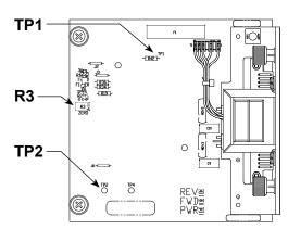
Low Current 120 V ac Relay Board Components
