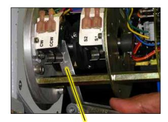
.030" (.75 mm) shim should be inserted between all levers and cams when setting switches.
