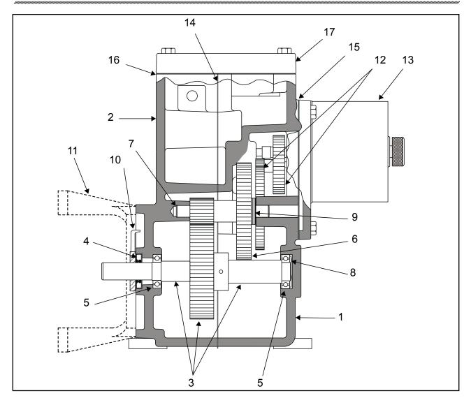
TYPICAL ACTUATOR COMPONENTS FOR MODELS 11-1\_\*
