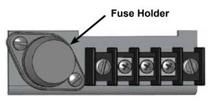
Turn the fuse holder CCW while pressing down. The fuse holder should spring loose when free. Remove the fuse holder from the actuator. Pull the fuse free from the holder. Replace the fuse with the same type (see table below) by pushing it into place.
