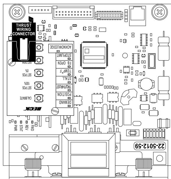
DCM-2 Board showing location of Thrust Wiring Connection
