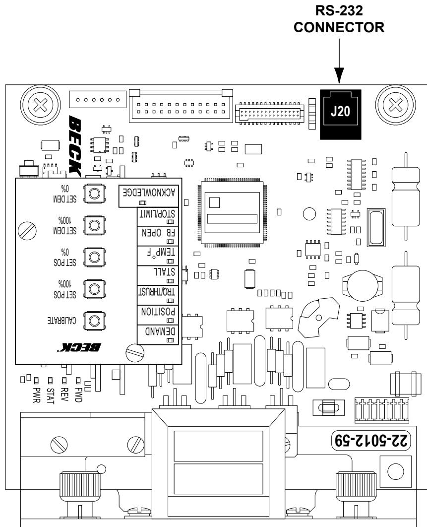
Location of RS-232 Connector on the DCM-2 Board
